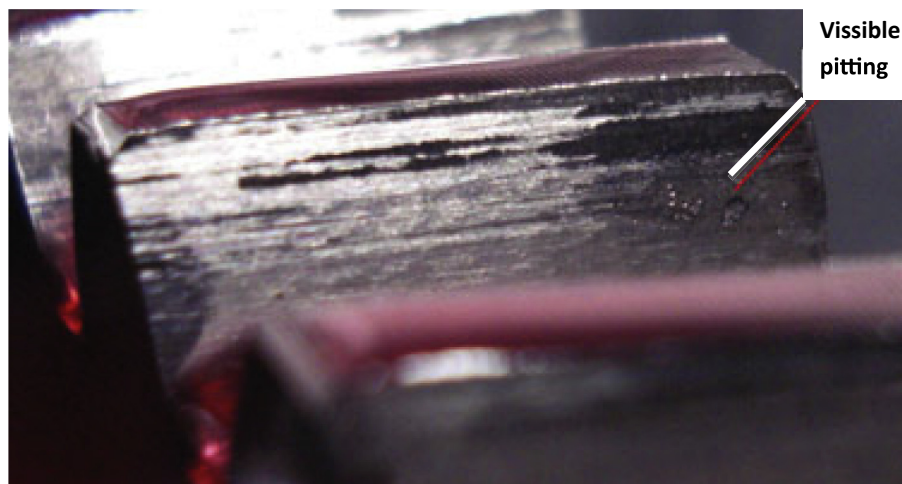
Fig. 13. Visible damage after test 2 [50].
