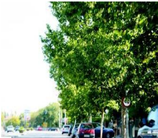
Figure 2.21 Bad Sign Positions (partially occluded signs)
