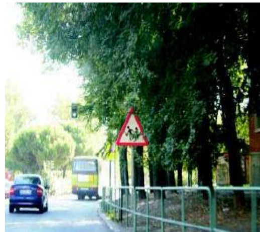
Figure 2.21 Bad Sign Positions (partially occluded signs)
