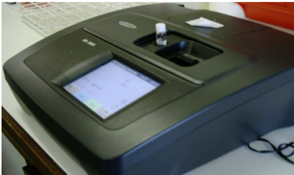
Appendix 6: DR 3800 SC Vis Spectrophotometer used to determine \text{H}_2\text{O}_2 concentration.
