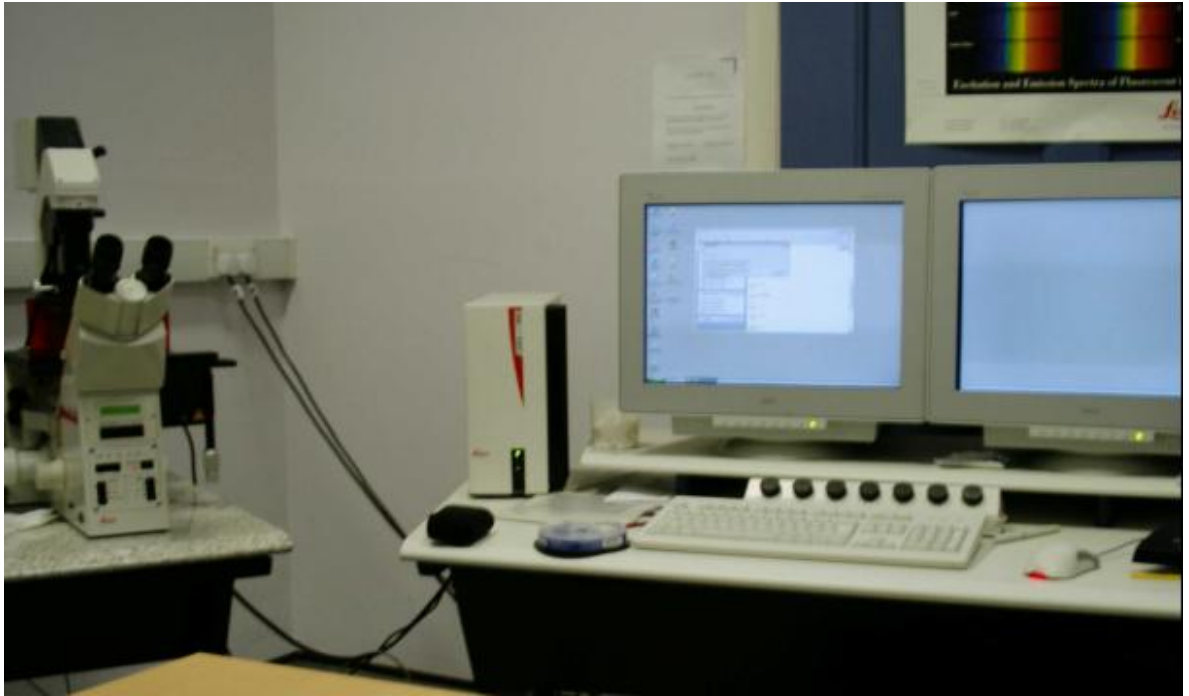
Appendix 9: True Confocal Scanner Leica TCS SP2 used for confocal microscopy work.
