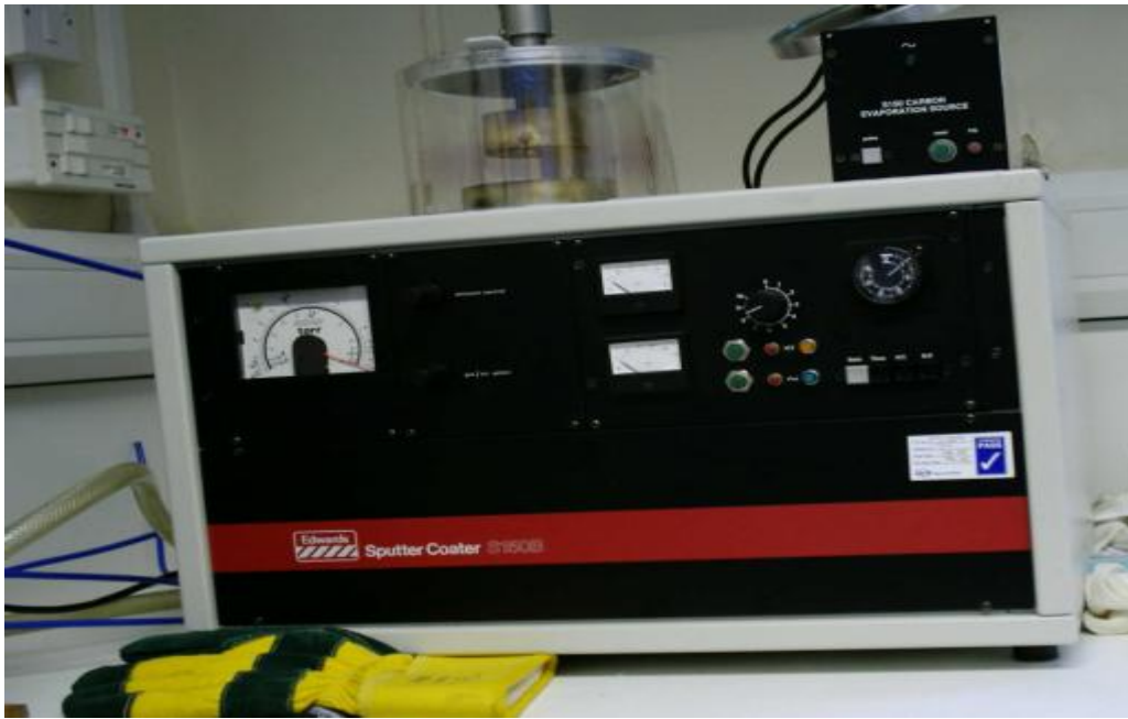
Appendix 8: Edwards Sputter Coater S150B for coating samples prior to electron microscopy and EDX analysis.
