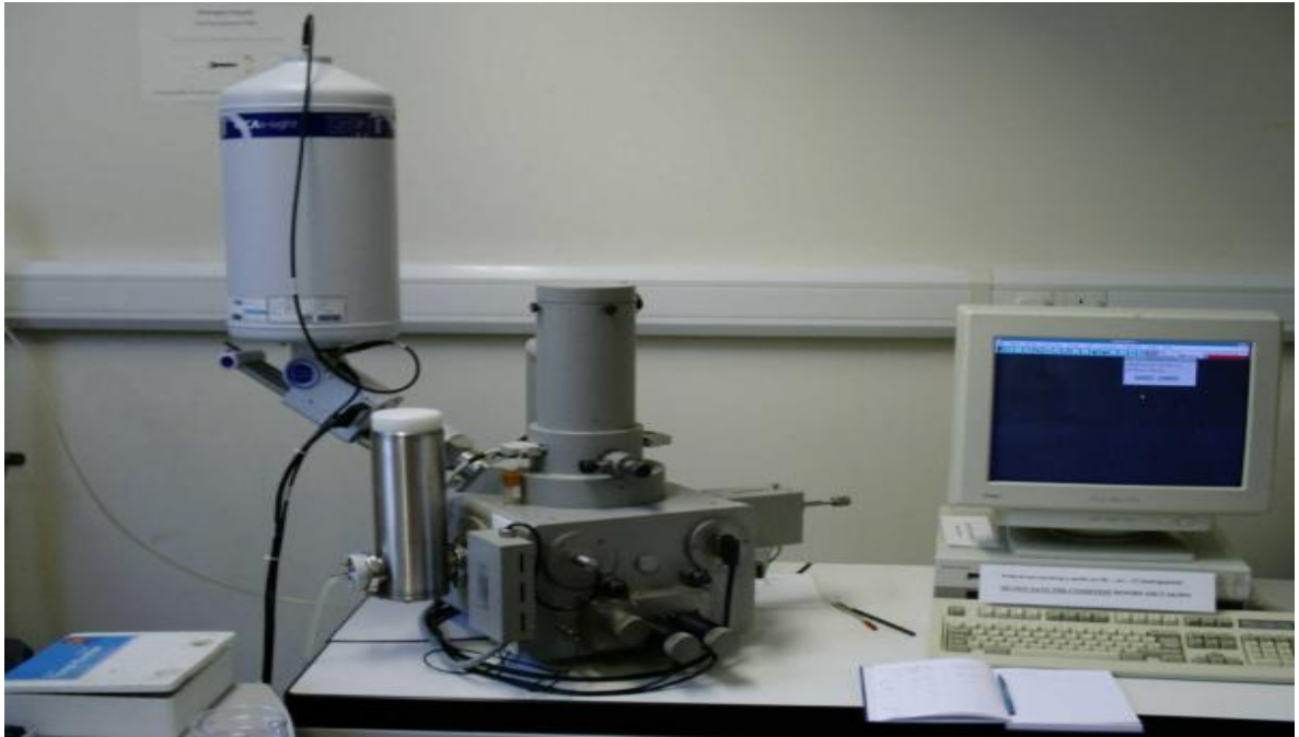
Appendix 7: Leica S430 for electron microscopy and Oxford Instruments INCA-Sight for EDX analysis.
