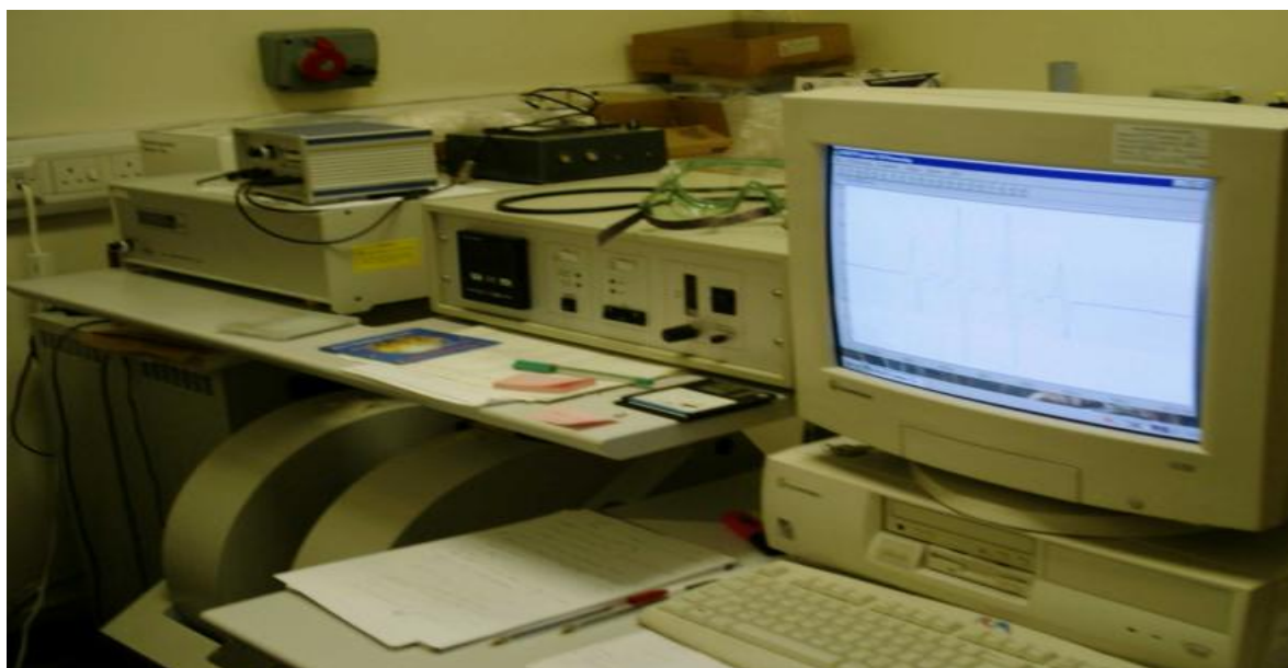
Appendix 5: Bruker EMX 6/1 EPR spectrometer used for hydroxyl radicals determination.
