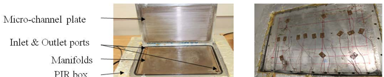
Figure 4: (a) Inner face of Test Rig (b) Thermocouple arrangement on plate
