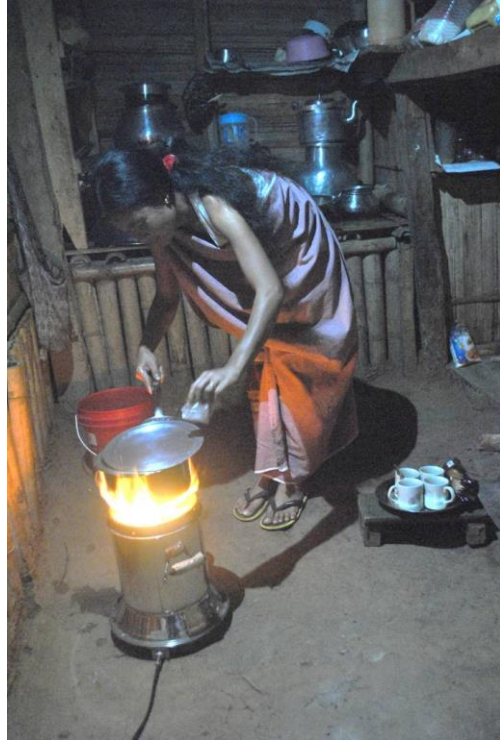
Figure 6: A user cooking food in a forced draft stove in a village in Meghalaya, India
