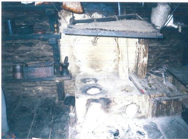
Figure 4: ICS customized by a user in a village in Bhutan depending on the need for smoking of food items
