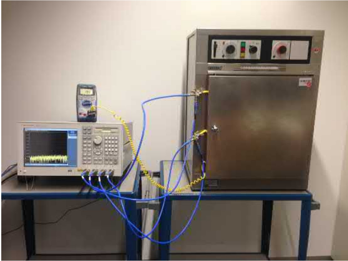
Figure 68 – Picture of measurement setup with heating cabinet
