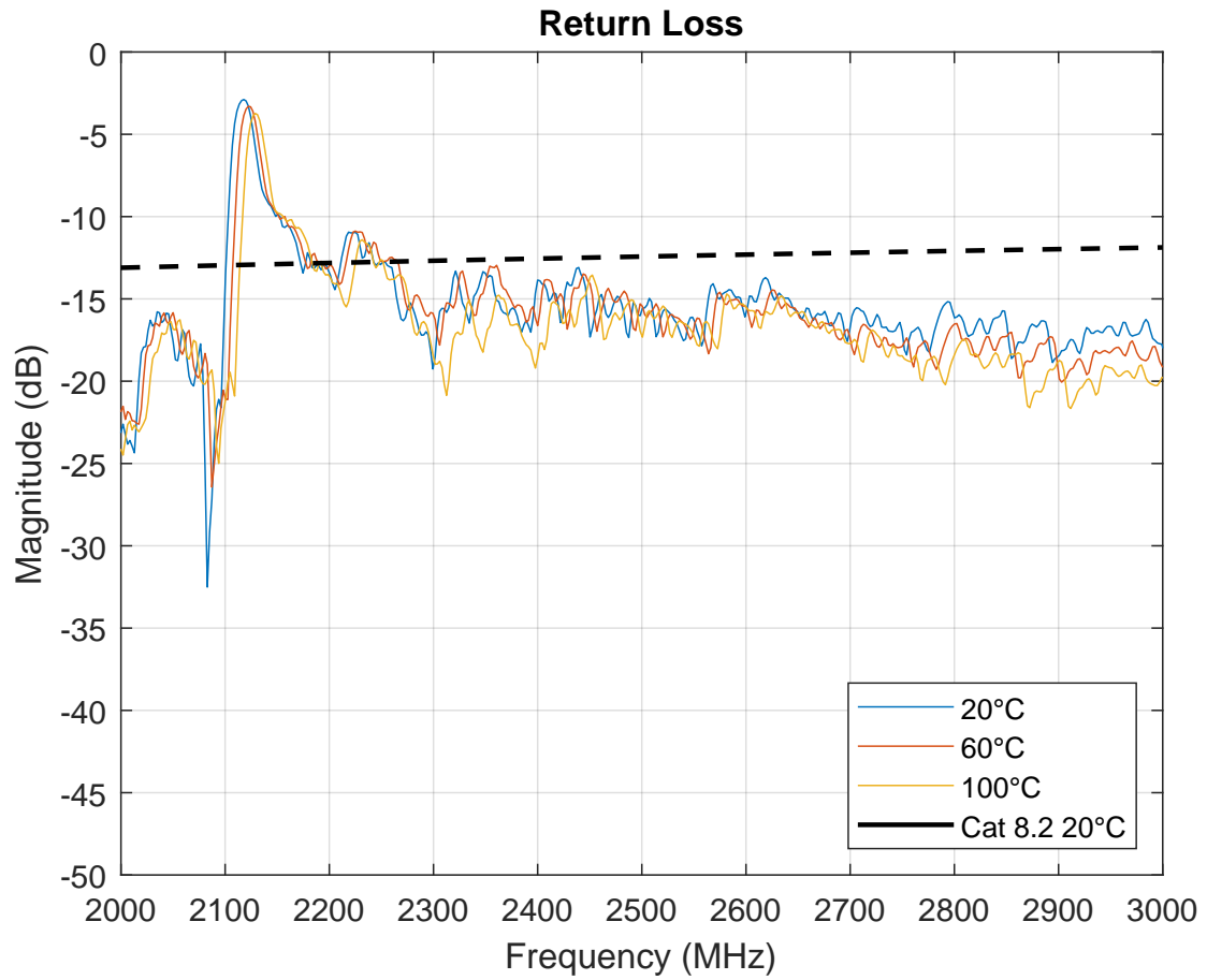
Figure 60 – RL of higher frequencies as a function of temperature and cable Cat 8.2
