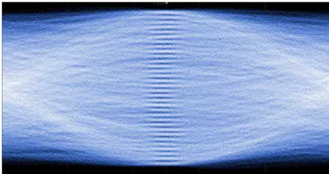
Figure 129 – 30 m - PAM 32 - 4.50 GBd - abscissa: 22 ps/div - ordinate: 80 mV
