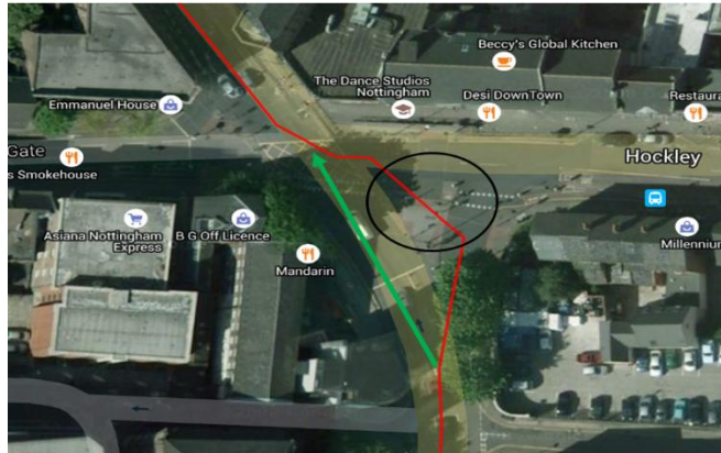
Figure 5-13: Error in Data set 1, green arrow is vehicle direction and black circle is the system error.
