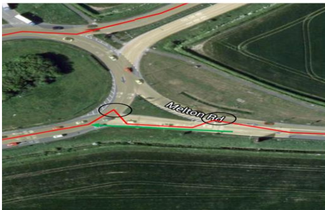
Figure 5-14: Error in Data set 2, green arrow is the vehicle direction and black circle is the system error.
