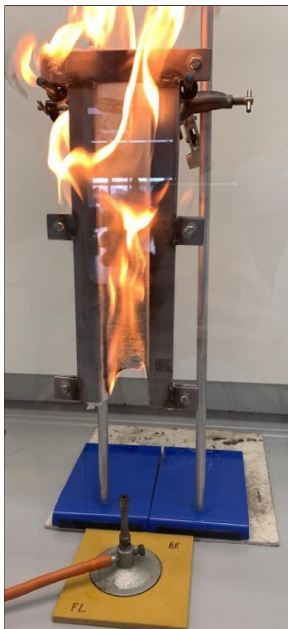
Figure 1. Vertical flammability test of viscose bandage.
