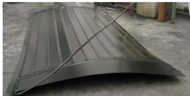
Figure 4.12: Deformed Rollbond Absorber with Extensive Fluid Channels (Collenz 2007a)
