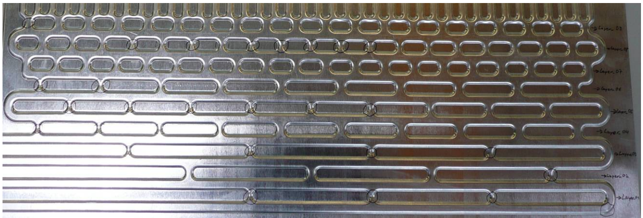
Figure E.2: Incompletely Inflated Channels in the Diverging Section
