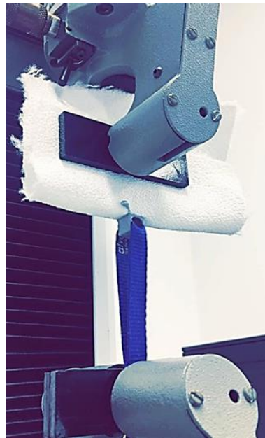
Figure 4 The tensile test method for 3D printed fabrics
