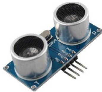
Figure 3. HC-SR04 ultrasonic sensor distance measuring module [19].
