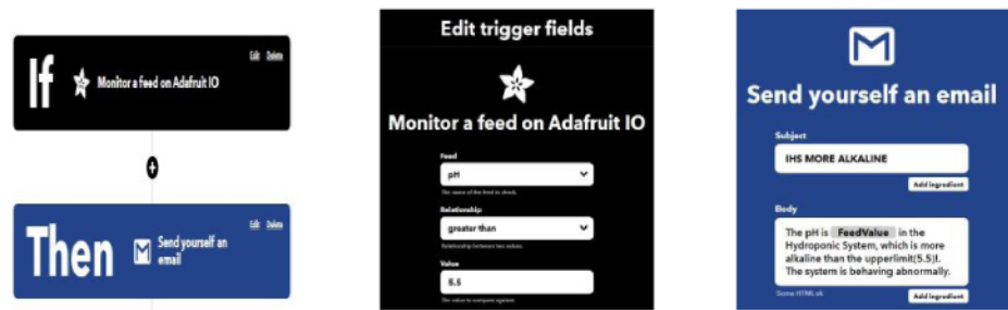
Figure 8. Setup at IFTTT’s end.
